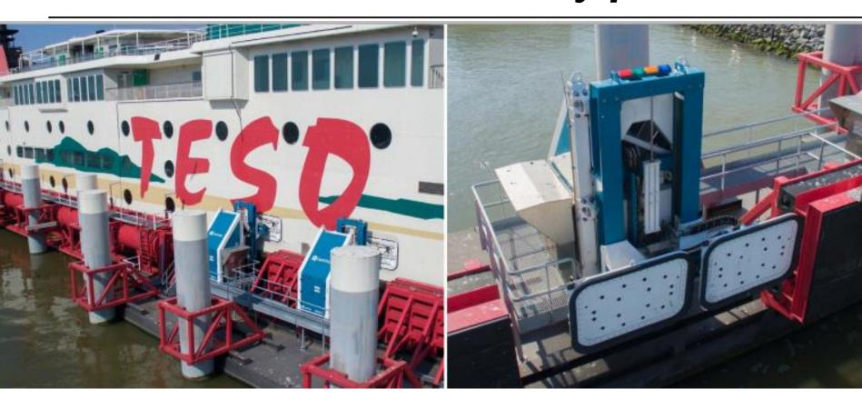
Every hour for 8 minutes the vessel is fixed to Cavotec **auto-mooring-system**. As during these minutes no energy is needed for thrust the ABC dual fuel engine - running at 100% - boosts the battery packs up to 90% state of charge.
