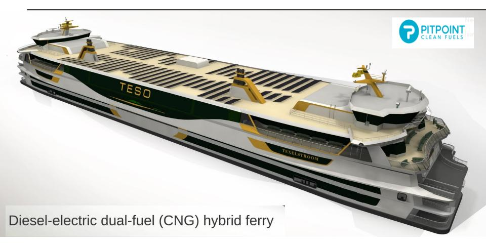
Compressed Natural Gas is clean burning fossil fuel which overall, compared to marine diesel fueled systems of similar propulsion capacity, produce 20% less CO2, 90% less SOx, 80% less NOx and 100% less particulate matter (PM). No smell from exhaust.
